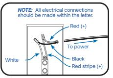
Connect the red stripe wire (+) of the LED strip to the red wire (+) of the power supply. Connect the white wire (-) of the LED strip to the black wire (-) of the power supply.
