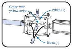
3 Connect the AC line to the black (line) and white (neutral) input wires of the power supply using 18-14 AWG (0.82-2.08 mm<sup>2</sup>) twist-on wire connectors. Properly ground (green wire with yellow stripe) power supply in accordance with National Electric Code (NEC) Article 600.
