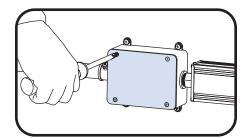
Tighten liquid-tight fittings and properly replace cover on junction box to ensure a water-tight seal. If not protected from the weather, the output connections may be sealed with electrical grade silicone.
