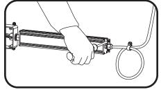
Mount Power Supply in a horizontal orientation with a minimum of one screw per mounting plate (two screws per power supply) with the base in contact with the mounting surface in accordance with the power supply spacing requirements described above.
