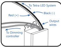
Connect the supply wire that is attached to the Tetra LED System to the red (+) and black (-) output wires of the power supply as outlined in the "Electrical Connections" section of your LED system's Installation Instructions.
