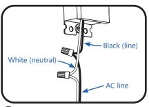
Connect the AC line to the black (line) and white (neutral) input wires of the power supply using 18-14 AWG (0.82-2.08 mm²) or 18-10 AWG (0.82-5.26mm²) twist-on wire connectors.
