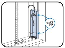
Mount the power supply with the base in contact with the mounting surface in an electrical enclosure with adequate dimensions to satisfy the power supply spacing requirements described above, and suitable for the installation environment. The power supply and electrical connections shall be protected from weather and not subject to saturation with water or other liquids. If not protected from the weather, the output and dimming connections may be sealed with electrical grade silicone.
