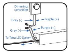
3 Connect the (+) purple and (-) gray wires of the Tetra Dimming Power Supply to the 0-10V dimming controller. Refer to the dimming controller installation instructions for specific connection information.
