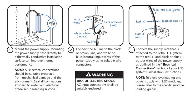
**NOTE:** For installation in Canada, a disconnect switch of appropriate rating needs to be placed within 29.5 feet (9 meters) of primary side of the power supply. The switch voltage rating shall not be less than the branch circuit voltage. The switch must also support twice the amount of input current.
