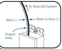
Connect the supply wire that is attached to the Tetra LED System to the red (+) and black or blue (-) output wires of the power supply as outlined in the "Electrical Connections" section of your LED system's Installation Instructions.
