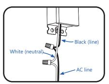
Connect the AC line to the black (line) and white (neutral) input wires of the power supply using 18-14 AWG (0.82-2.08 mm<sup>2</sup>) or 18-10 AWG (0.82-5.26mm<sup>2</sup>) twist-on wire connectors. Properly ground power supply in accordance with National Electric Code (NEC) Article 600.
