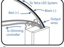
Connect the supply wire that is attached to the Tetra LED System to the red (+) and black (-) output wires of the power supply as outlined in the "Electrical Connections" section of your LED system's Installation Instructions.
