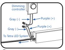
3 Connect the (+) purple and (-) gray wires of the Tetra Dimming Power Supply to the 0-10V dimming controller. Refer to the dimming controller installation instructions for specific connection information.
