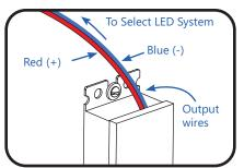
Connect the supply wire that is attached to the Select LED System to the red (+) and blue (-) output wires of the power supply as outlined in the "Electrical Connections" section of your LED system's Installation Instructions.
