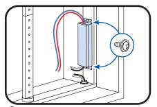
Mount the power supply. Mounting the power supply base directly to a thermally conductive installation surface can improve thermal performance.
