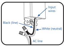
Connect the AC line to the black (2)(line) and white (neutral) input wires of the power supply using suitable wire connectors.
