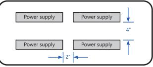
2 If installing multiple power supplies, keep them at least 2" (50.8mm) apart end to end and 4" (101.6mm) apart along the sides.
