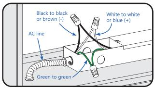
Wire AC line to power supplies in accordance with the applicable local, state, and country electrical codes. Connect black to black or brown, white to white or blue, and green to green using 18 AWG (0.82mm²) wire connectors.
