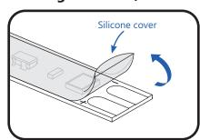
At the cut end, carefully peel back the silicone cover over the soldering pads. Make sure not to remove the silicone over the LED.
