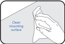
Mounting surface must be free of dust, dirt or grease. Clean mounting surface with alcohol before installation and allow to dry.
