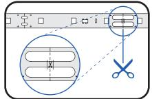
Measure and cut Tetra® flexible tape to the desired length using scissors. Cut only on the scissor markings and stay within the limit lines.
