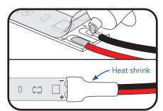
6a) Seal the soldering points with electrical silicone. Replace the silicone cover and secure it by shrinking a piece of 1/4" heat shrink over the end.
