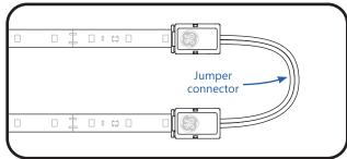
7 If necessary, join two strips together using a jump connector or a soldered wire connection. Follow steps 4b-6b for each end of the jump connection, or 4a-6a for each end of the soldered wire connection.
