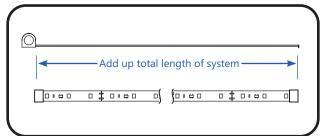
1 Add up total footage of the system to determine the appropriate number of 12VDC Class 2 Tetra® power supplies to use based on the **Power Supply Loading** chart on last page.
