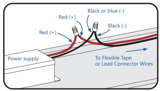
3 Connect the red wire (+) of the LED system to the red wire (+) of the power supply. Connect the black wire (-) of the LED system to the black or blue wire (-) of the power supply.
