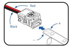
Partially remove the tape backing on the end to be connected. Align red lead with the (+) contact on the tape and the black lead with the (-) contact. Fully insert the tape into the open end of the tape guide with the LEDs facing the cover.
