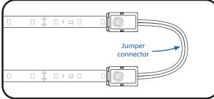
7 If necessary, join two strips together using a jump connector or a soldered wire connection. Follow steps 4b-6b for each end of the jump connection, or 4a-6a for each end of the soldered wire connection.
