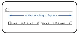
Add up total footage of the system to determine the appropriate number of 12VDC Class 2 Tetra\* power supplies to use based on the Power Supply Loading chart on last page.
