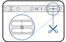
2 Measure and cut Tetra\* flexible tape to the desired length using scissors. Cut only on the scissor markings and stay within the limit lines.
