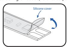
4a) At the cut end, carefully peel back the silicone cover over the soldering pads. Make sure not to remove the silicone over the LED.
