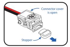
(4b) Check the connector for cosmetic issues. Open the cover. Remove the stopper from the tape guide.
