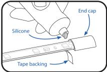
Peel away a portion of the tape backing at cut end. Press fit an end cap fully to the open end and apply electrical grade silicone (see examples above).
