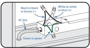
Wire AC line to power supplies in accordance with the applicable local, state, and country electrical codes.
