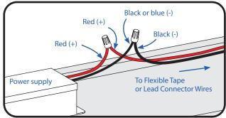
Onnect the red wire (+) of the LED system to the red wire (+) of the power supply. Connect the black wire (-) of the LED system to the black or blue wire (-) of the power supply.
