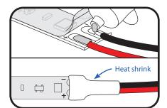
6a) Seal the soldering points with electrical silicone. Replace the silicone cover and secure it by shrinking a piece of 1/4" heat
