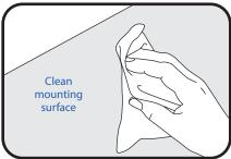
Mounting surface must be free of dust, dirt or grease. Clean mounting surface with alcohol before installation and allow to dry.
