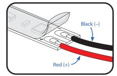
Using UL certified 18AWG wire, solder a red wire to the (+) pad and a black wire to the (-) pad.
