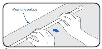
8 Remove tape backing and stick Tetra\* flexible tape in place. Ensure the tape is firmly attached.
