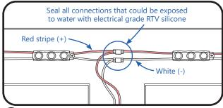
Connect LED strips using in-line (IDC) connectors or twist-on wire connectors.
