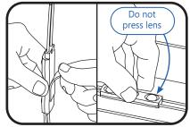
Remove tape backing and stick LED modules into place. When using tape apply approximately 15 psi pressure on the module (avoid the lens dome surface) for 5 seconds, full bonding strength after 24 hours. Continue until you have reached the end of the strip.
