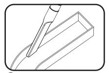
Before you begin, clean surfaces and remove all debris from the inside of the channel letter. Clean the surfaces with a 50:50 mixture of isopropyl alcohol (IPA) and water and let dry.
