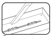
Remove all debris from the inside 6 of the channel letter and replace the sign face.
