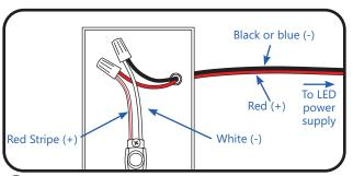
4 Connect the red stripe wire (+) of the LED strip to the red wire (+) of the power supply. Connect the white wire (-) of the LED strip to the black or blue wire (-) of the LED power supply.
