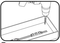
Drill a 1/4-inch (6.4 mm) hole near the LED strip and grommet the hole for supply wire access.
