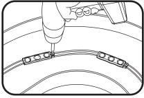
Use rivets, screws, or electrical grade RTV silicone to secure at least every third LED module within the channel metal screws, 1/8-inch (3.2 mm) rivets, or electrical grade RTV silicone.
