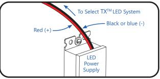
Run a wire from the LED Power Supply to each channel letter and connect to the first LED module on the strip.
