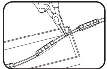
Measure and cut Select TX™ LED strip to the appropriate length for each letter. Cuts can be made between any of the modules.
