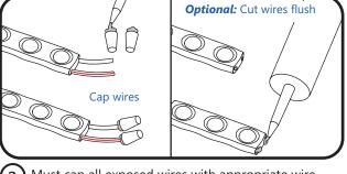
Must cap all exposed wires with appropriate wire connectors and seal with electrical grade RTV silicone.
