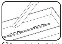
6 Remove all debris from the inside of the channel letter and replace the sign face.
