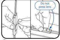
3 Remove tape backing and stick LED modules into place. When using tape apply approximately 15 psi pressure on the module (avoid the lens dome surface) for 5 seconds, full bonding strength after 24 hours. Continue until you have reached the end of the strip.
