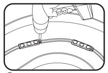
4 Use rivets, screws, or electrical grade RTV silicone to secure at least every third LED module within the channel letter. Use #6 (M3) or #4 pan headed metal screws, 1/8-inch (3.2 mm) rivets, or electrical grade RTV silicone.
