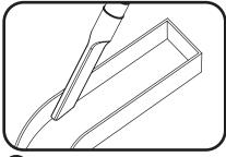
D Before you begin, clean surfaces and remove all debris from the inside of the channel letter. Clean the surfaces with a 50:50 mixture of isopropyl alcohol (IPA) and water and let dry.
