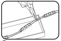
2 Measure and cut Select TX<sup>™</sup> LED strip to the appropriate length for each letter. Cuts can be made between any of the modules.
