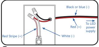
Connect the red stripe wire (+) of the LED strip to the red wire (+) of the power supply. Connect the white wire (-) of the LED strip to the black or blue wire (-) of the LED power supply.
