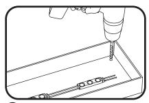
5 Drill a 1/4-inch (6.4 mm) hole near the LED strip and grommet the hole for supply wire access.
