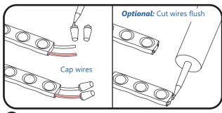
2 Must cap all exposed wires with appropriate wire connectors and seal with electrical grade RTV silicone.
