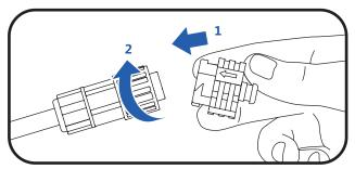
4 Insert an end cap into the female connector on the last luminaire in the run, and twist the end cap clockwise to secure.
