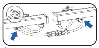
Optional: Secure the cables using the optional cable clamp accessory.
