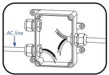
Using a Listed ½" Fitting suitable for the wiring method and appropriate environmental rating for the installation, bring the branch circuit conductors into the junction box.
