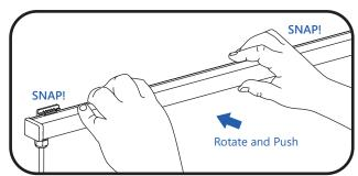
Press the luminaire into its mounting clips so that the male connector is oriented towards the intended electrical supply. *TIP:* Align luminaire on one side of the mounting clips; then rotate the luminaire until it snaps into other side of the mounting clips.
