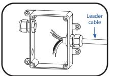
Insert the leader cable into the cable gland and tighten the cable gland bushing nut to secure the power cord.
