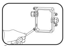
1 Secure the junction box to a mounting surface using four (M4) self-tapping flathead screws adjacent to the supply side of the intended run of luminaire.
