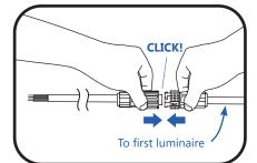
2 Insert the female connector of the leader cable so that it fully engages the male connector of the first luminaire in the run as indicated by hearing a click.
