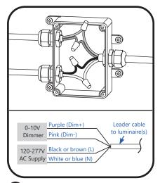
7 Connect the DIM + (purple) to the incoming dimmer circuit +. Connect the Dim – (pink) to the incoming dimmer circuit –.
