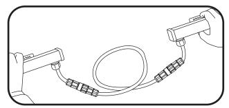
Use a jumper cable to connect luminaires if the distance between them is too long.
