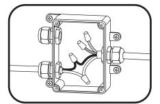
AC Supply Wire Connections Inside the junction box, connect the line and neutral wires of the AC supply source to the line (black or brown) and neutral (white or blue) wires of the leader cable using suitable wiring connectors. If 0-10V dimming will not be used, cap the dimming wires (purple and pink) with suitable wiring connectors. Do not connect the dimming wires together or to line, neutral, or ground. If 0-10V dimming will be used, proceed to Step 6.
