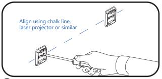
Secure each luminaire mounting clip to a rigid flat mounting surface using two #10 (M5) self-tapping flathead screws along the intended run of luminaire.
