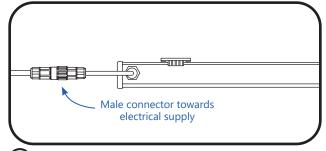
Place the luminaire on the surface with the male connector oriented towards the intended electrical supply.
