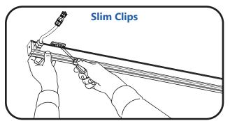
Using a screwdriver, gently pry the luminaire out of the mounting clips.
