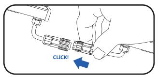
Remove end cap from the female connector. Insert the male connector to the female connector. Make sure the connector is fully engaged as indicted by hearing a click.
