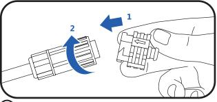
4 If not already covered, insert an end cap into the female connector, and twist the end cap clockwise to secure.
