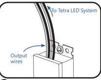
3 Connect the supply wire that is attached to the Tetra LED System to the red (CH1 +) and red/white (CH1 -), or blue (CH2 +) and blue/ white (CH2 -) output wires of the power supply as outlined in the "Electrical Connections" section of your LED system's Installation Instructions.
