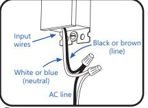
2 Connect the AC line to the black (line) and white (neutral) input wires of the power supply using suitable wire connectors.
