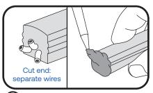
6 For cut end, manually untwist and separate wires to avoid shorts. Seal light engine end with electrical grade silicone. Clean excess silicone.
