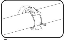
6 Secure light guide by twisting tie-wire around the mounting clip and light guide.
