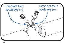
9 Use twist-on wire connectors to join wires together.
