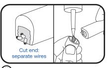
For cut end, manually untwist and separate wires to avoid shorts. Fill cap with electrical grade silicone and push cap on the end to seal. Clean excess silicone.
