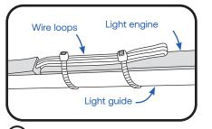
Wires between light guide segments can be folded behind the light guide and attached with clear zip ties. Zip ties should wrap around outside light guide.
