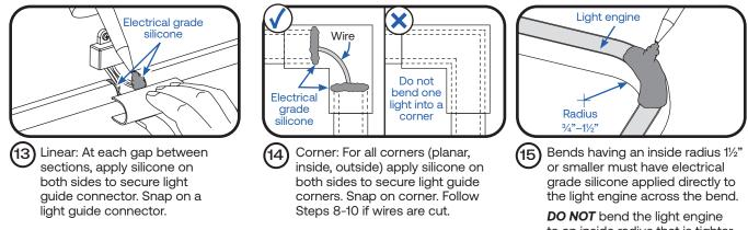
to an inside radius that is tighter than 3/4 in. (19mm).
