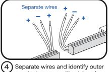
Separate wires and identify outer conductors as positive (+) and middle conductors as negative (–). Strip ends back 0.5 in. (13mm).
