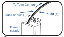
Run a wire from the power supply to a section of Tetra Contour. Power supply connection must be completed in an acceptable UL/NEMA enclosure. Power supply loading is described in the power supply installation instructions.
