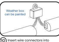
weather box. Fill with electrical grade silicone and close box. Weather box can be mounted using #8 (M3) screws.
