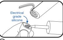
12) For uncut end, fold wire over Tetra Contour. Fill the end cap with silicone and push cap on the end to secure. Clean excess silicone.
