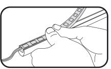
3 Push the light engine segments down into the light guide.
