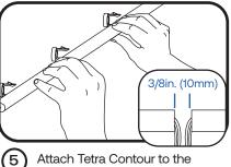
Attach Tetra Contour to the mountingclips, leaving a 3/8 in. (10mm) gap between sections to allow for expansion or contraction.
