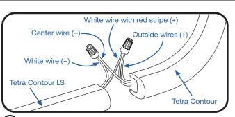
2 Splice the white wire with red stripe (+) of Tetra Contour LS to the two outside wires (+) of Tetra Contour and splice the white wire (-) of Tetra Contour LS to the center wire (-) of Tetra Contour.
