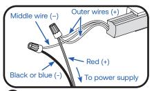
Connect the two outer wires (+) from the LED strip to the red wire (+) of the power supply. Connect the middle wire (-) from the LED strip to the black or blue wire (-) of the power supply. Grounding and bonding must be done in accordance with National Electrical Code (Article 600). See power supply instructions.
