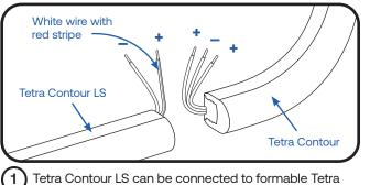
Tetra Contour LS can be connected to formable Tetra Contour for custom shapes. Separate wires and identify conductors as positive (+) and negative (–). Strip ends back 0.5 in. (13mm).
