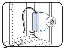
Mount the power supply. Mounting the power supply base directly to a thermally conductive installation surface can improve thermal performance.
