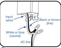
2 Connect the AC line to the black or brown (line) and white or blue (neutral) input wires of the power supply using suitable wire connectors.
