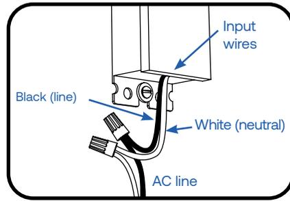
2 Connect the AC line to the black (line) and white (neutral) input wires of the power supply using suitable wire connectors.
