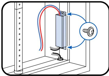
1 Mount the power supply. Mounting the power supply base directly to a thermally conductive installation surface can improve thermal performance.
