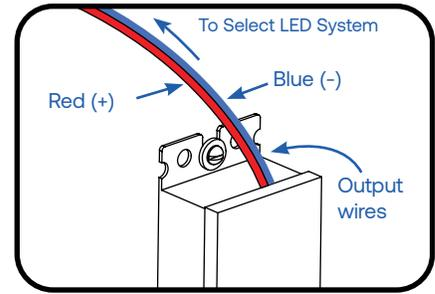
3 Connect the supply wire that is attached to the Select LED System to the red (+) and blue (-) output wires of the power supply as outlined in the “**Electrical Connections**” section of your LED system’s Installation Instructions.
