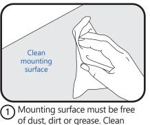
of dust, dirt or grease. Clean mounting surface with alcohol before installation and allow to dry.
