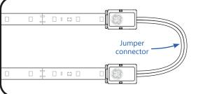
If necessary, join two strips together using a jump connector or a soldered wire connection. Follow steps 4b-6b for each end of the jump connection, or 4a-6a for each end of the soldered wire connection.
