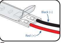
Using UL certified 18AWG wire, solder a red wire to the (+) pad and a black wire to the (-) pad.
