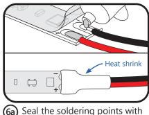
Seal the soldering points with electrical silicone. Replace the silicone cover and secure it by shrinking a piece of 1/4" heat shrink over the end.
