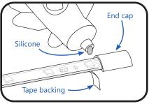
Peel away a portion of the tape backing at cut end. Press fit an end cap fully to the open end and apply electrical grade silicone (see examples above).
