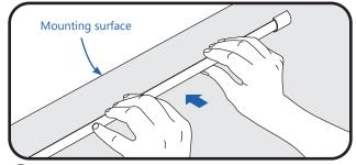
8 Remove tape backing and stick Tetra<sup>®</sup> flexible tape in place. Ensure the tape is firmly attached.
