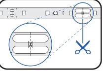
Measure and cut Tetra<sup>®</sup> flexible tape to the desired length using scissors. Cut only on the scissor markings and stay within the limit lines.
