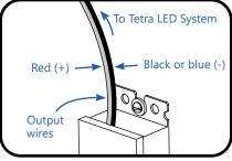
Connect the supply wire that is attached to the Tetra LED System to the red (+) and black or blue (-) output wires of the power supply as outlined in the "Electrical Connections" section of your LED system's Installation Instructions.
