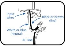
Connect the AC line to the black or brown (line) and white or blue (neutral) input wires of the power supply using suitable wire connectors.
