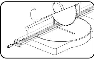
2 If it is necessary to cut the lightbar for a better fit, the cutting resolution is 3 inches (76.2 mm). Cut the lightbar as necessary to fit the application. Only cut the PCBA from the back to the front. DO NOT cut from the LED side to the back.
