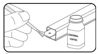
Apply and seal the cut end of the LED board with a brush-on conformal coating such as MG Chemicals 419D, Humiseal 1B73, or Electrolube APL. Allow at least 10 minutes to dry.
