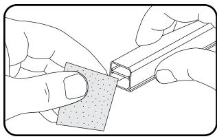
3 Clean debris from extrusion cut end with the sandpaper and avoid sanding the edge of the LED board.
