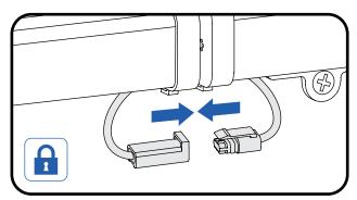
Mate the male and female connectors of each adjacent light bar while ensuring the connectors are oriented in the same direction. DO NOT attempt to mate upside down or otherwise exert excessive force on the light bar connectors. Be sure that the retaining clip of the connectors are fully engaged and locked together as indicated by a click. Attach jumper cables as needed to work around any obstacles, corners or separations. DO NOT pull on the wires when un-mating the connectors.
