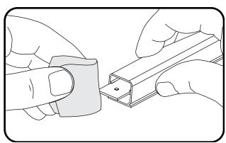
Pull out the LED board gently and clean and deburr the cut end with a cloth or other appropriate tool. Be careful not to damage the dielectric, and to ensure no copper from the trace is making contact with the PCB assembly substrate. Finally, shake or blow out any dust and debris from the extrusion.
