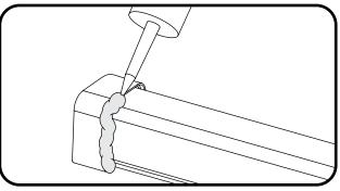
Apply electrical grade RTV silicone around the outside circumference of the end cap. Ensure that the silicone completely seals the joint between the end cap and light bar.
