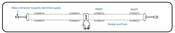
Press each light bar into its mounting clips and slide it into the adjacent light so that the alignment features in the end caps mate with each other.
