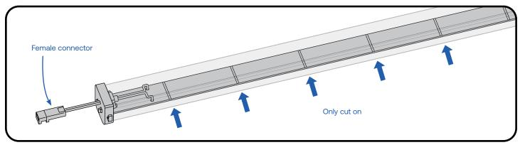
For planning the layout, measure the desired length to be lit and divide by the Light Bar Length (L) in the table above to determine the required quantity of light bars. If it is necessary to cut the light bar for a better fit, the cutting resolution is 3 inches (76.2 mm).
