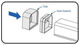
Push the GELLCAP seal gasket and cap over the cut end of the light bar.
