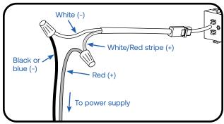
Using twist-on wire connectors, connect the white/red stripe wire (+) from the light bar to the red wire (+) of the power supply. Connect the white wire (-) from the light bar to the black or blue wire (-) of the power supply.
