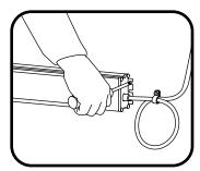
Mount Power Supply with a minimum of one screw per mounting plate (two screws per power supply) with the base in contact with the mounting surface in accordance with the power supply spacing requirements described above.
