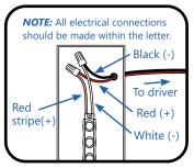
Connect the supply wire that is attached to the Tetra LED System to the red (+) and black (-) output wires of the power supply as outlined in the "Electrical Connections" section of your LED system's Installation Instructions.
