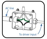
Inside the junction box, connect the line, neutral, and ground wires of the AC supply source to the line (black), neutral (white), and ground (green wire with yellow stripe) wires of the leader cable using suitable wire nuts. Install the junction box cover.
