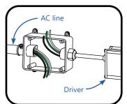
Run AC supply and power supply leader cable into a junction box suitably approved and rated for the application through the appropriate fittings.
