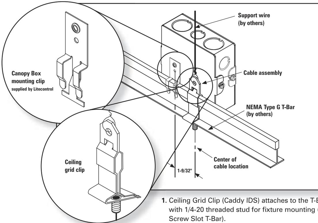
1. Ceiling Grid Clip (Caddy IDS) attaches to the T-Bar at each feed cable location with 1/4-20 threaded stud for fixture mounting (Caddy IDS 9.5 attaches to a Screw Slot T-Bar).
