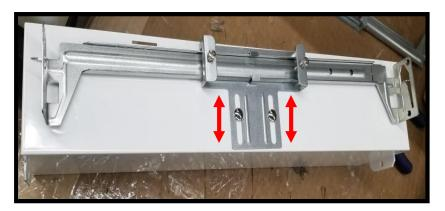
Bar hanger position can be adjusted by loosening the screws and sliding the bracket up/down
