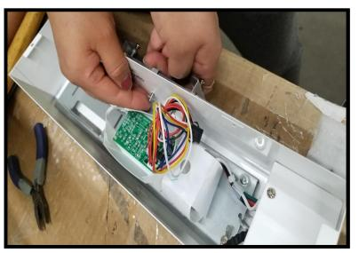
Using the screws and wingnuts secure the bar hanger to the housing
