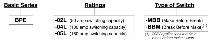
Example: **BPE-02L-MMB** (50 amp make-before-break bypass switch)
