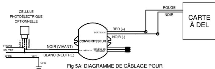
Fig 5A: DIAGRAMME DE CÂBLAGE POUR PROJECTEUR FSL
