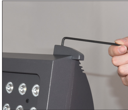
2. Install Barn Door Hinge with (8) 8-32 x 1/2" screws.
