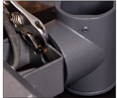
3. Torque nuts to 10 foot-pounds.
