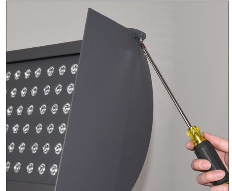
3. Install Barn Door Flaps with (8) 10-32 x 3/8" screws and #10 washers.
