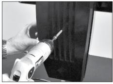
Attach cover and tighten with 3/16" hex key or drill bit.
