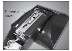
Avoid running wires over electronic driver to eliminate any chance of pinching wires.
