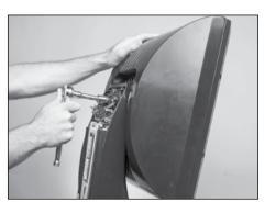
**9.** Fixture head has a +30° to -5° tilt allowance for aiming. Loosen (2) bolts with 3/16" hex wrench. to adjust tilt on head. When head is at selected angle, tighten the two bolts sufficiently to eliminate unwanted movement.
