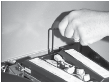
10. Install speed mount retaining screw and tighten securely using 3/16" hex wrench.
