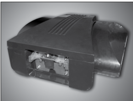
13. Speed Mount Adapter Plate for Downlight – A down luminaire can be converted to an up luminaire by removing the Speed Mount adapter Plate, rotating it 180° and reconnecting it to the back of the arm mount. The plastic connector always faces down on the Speed Mount Adapter Plate.
