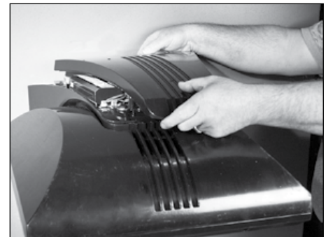
12. Ensure no wires are routed over the top of driver(s) to avoid pinching wires. Replace arm cover and tighten securely using 3/16" hex wrench.
