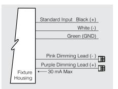
0-10V Dimming: Driver has a 0-10V dimming interface with a dimming range of 10-100%. The driver is compatible with most controls systems including NX Lighting Controls. Note: Not compatible with current sourcing dimmers. Controls compatible via purple and pink dimming leads.
