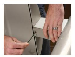
**12.** Remove splice cover screw. Hook top of splice cover into opening in arm and swing into place. Replace splice cover screw.
