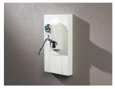
2. Mount Speed Mount to cover plate with 2 bolts. Pull wiring through cover plate and Speed Mount. Cover plate hangs from the top of wall mounting bracket and is secured with (2) 10-32 screws at bottom of cover plate. Secure screws with B" hex wrench. Mount Access Cover to Cover Plate. Secure with B" hex wrench.
