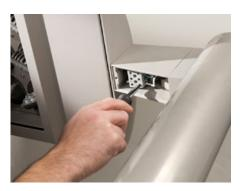
**11.** Tighten terminal block screws with a flat blade screwdriver.
