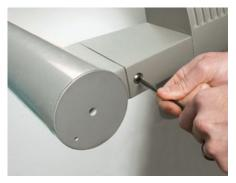
**1.** With J" hex wrench, remove embedded top bolt.
