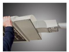
1. Optional horizontal slip-fitter arm is available for mounting to a 1J" to 2" pipe-size mounting end (1D" to 2C" OD). The casting has a ±5° adjustment to accommodate davit arms that are not horizontal.
