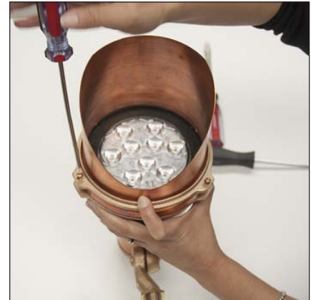
19. Place LED light engine and shield into body spinning, Slide clamping ring back onto body spinning. Re-attach backup ring to hold shield in place
