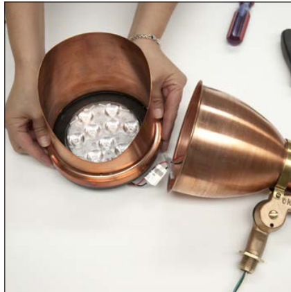
18. Insert shield onto LED light engine.
