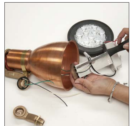
13. Attach electronic driver bracket to socket mounting plate.
