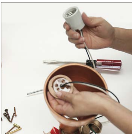
7. Pull socket and black and white leads from socket mounting plate and body spinning. Discard socket.
