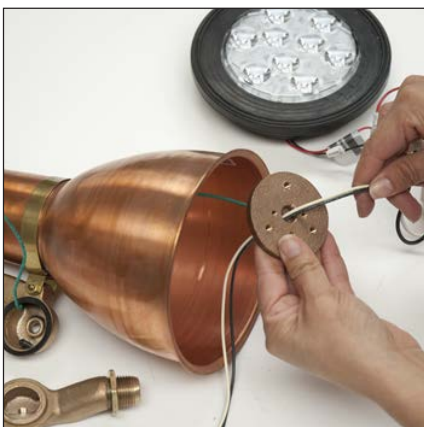
11. Insert the white and black leads from the electronic driver upgrade kit through the socket mounting plate, body spinning and swivel arm.
