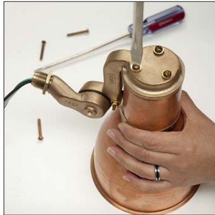
5. Remove screws connecting swivel arm to socket mounting plate and set aside.
