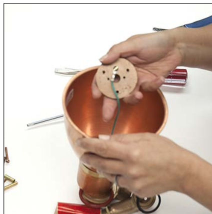
8. Avoid removing green grounding lead from socket mounting plate.
