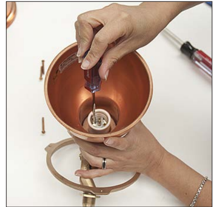
2. Remove screws holding socket to socket mounting plate and discard.
