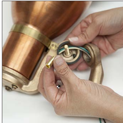
15. Run wire leads through swivel stem. Insert swivel arm screw, place sleeve over screw and seal gasket and swivel stem onto swivel arm.
