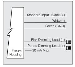
0-10V Dimming: Driver has a 0-10V dimming interface with a dimming range of 10-100%. The driver is compatible with most controls systems including NX Lighting Controls. Note: Not compatible with current sourcing dimmers. Controls compatible via purple and pink dimming leads.
