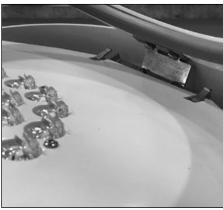
**3.** Hang bezel plate. Orientation determined by location of slots.
