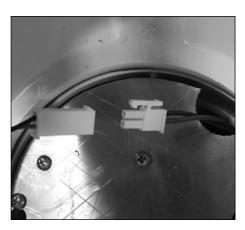
**5.** Connect quick-disconnect from driver assembly to bezel assembly.
