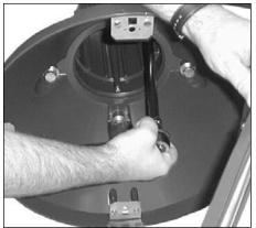
**1.** Install fixture to arm with lock washers & nuts Tighten to 20 ft-lbs. Make sure fixture aligns with arm with "hinge" side of fixture towards pole.
