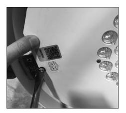
**6.** Secure bezel assembly with 1/4 turn fastener.
