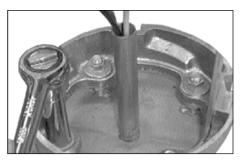
Tighten the upper nuts using a 9/16" deep socket
