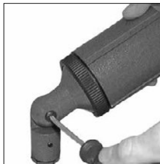
3. Adjust angle using swivel screw. Retighten after adjustments.
