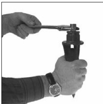
1. Tighten coupling onto mounting device. (See KIM Installation Instructions for Low Voltage Mounting Options, part no. 95488.)
