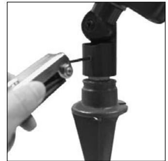
4. Loosen set screw, adjust fixture rotation, and tighten set screw.
