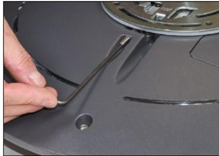
**7.** Tighten the set screw on the side of the fixture (this will allow latch to be temper proof).
