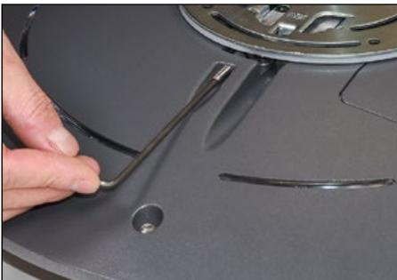
**1.** Loosen the set screw on the side of the fixture.
