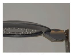
Optional horizontal slip-fitter arm is available for mounting to a 1-1/4" to 2" pipe-size mounting end (1-5/8" to 2-3/8" OD). The casting has a ±5° adjustment to accommodate davit arms that are not horizontal.
