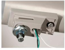
**5.** Thread top bolt through flat washer and shoulder washer, and bottom bolt through flat washer into pole backing plate inside pole.
