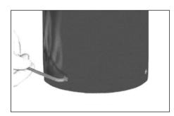
7. Tighten two 3/8" set screws at the bottom of the pole using a 3/16" hex key.
