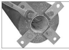
2. Install four anchor plates using 15/16" wrench with four 5/8-11 hex head bolts povided. Position the anchor plates straight from center on round bollards (see plan view below).
