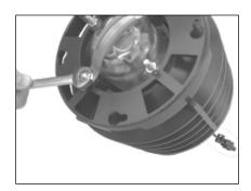
**6.** Using 7/16" wrench, remove two 1/4-20 nuts securing retaining cap.
