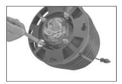
Continue to remove four 1/4-20 nuts securing louver stsck. Remove louver stack and set aside.
