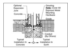
**4.** Make final adjustments to level bollard by turning the bottom nuts on the anchor bolts. The bollard must have full contact with concrete foundation by grouting. Mounting hardware must
