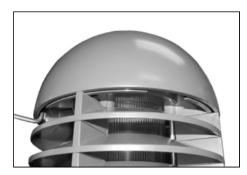
**13.** Locate two top cap screws (180° apart) and place into keyhole slots in louver cap. Tighten cap by turning counter-clockwise. After top cap is locked in place, tighten two top cap button hhead screws using 5/32" allen wrench.
