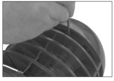
**5.** Locate two 1/4-20 button head cap screws (180° apart) concealed 3/4" up under top cap. Loosen, do not remove, screws with 5/32" allen wrench. Turn cap clockwise and lift up to remove.
