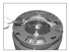
**12.** Using 7/16" wrench, attach louver cap and retaining strap to louver stack using 1/4-20 nuts.
