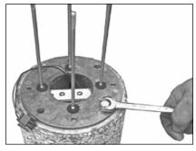
**9.** Pull quick-disconnect from driver assembly through hole in center of mounting plate. Use 7/16" wrench, secure mounting plate to riser with four 1/4-20 hex bolts provided.
