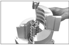
**13.** Louver installation: Install two louver stacks without retainer bracket first, 180° apart by sliding onto the tension rods. Next, install the two louver stacks containing the retainer brackets 180° apart by sliding onto the tension rods.
