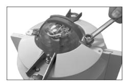
**15.** Using 7/16" wrench, replace retaining strap and tighten with two 1/4-20 nuts.
