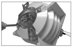
7. Using 7/16" wrench, remove four 1/4-20 hex nuts securing louver stack. Slide louver stacks off rods and set aside.
