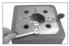
**10.** Using 7/16" wrench, install mounting plate with four 1/4-20 bolts provided.
