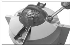
**6.** Using 7/16" wrench, remove two 1/4-20 nuts securing retaining strap. Rermove retaining strap and glass globe.
