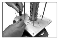
**11.** Join the disconnect plugs between driver assembly and optical assembly. Tuck extra wire into riser ensuring no wires get pinched during next step.
