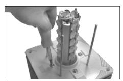
**12.** Using a flat blade screwdriver re-ttach the bottom casting/optical assembly to the mounting plate with four 1/4-20 screws.
