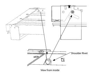
5) Close Jaw by rotating up, lift up & slide Jaw forward install optional security screw (if one is present).
