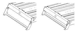
Insert rivet head through keyhole of Jaw pivot track (both sides).
