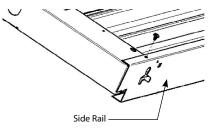
3) Install VersaBay<sup>®</sup> End Jaw, engaging shoulder rivet in slotted opening in side rails as shown below.
