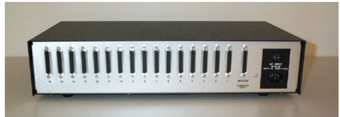
Rear of Multiplexer
