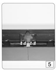
Ensure both housing units line up properly with minimal of gap between them and fully tighten all screws. Do not over tighten the screws or damage to the housing screw bosses could occur.
