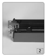
Slide the mating plate into the housing opening. Push the mating plate in till the slots of the mating plate engage the rails in the housing and the plate bottoms out on the screw bosses.
