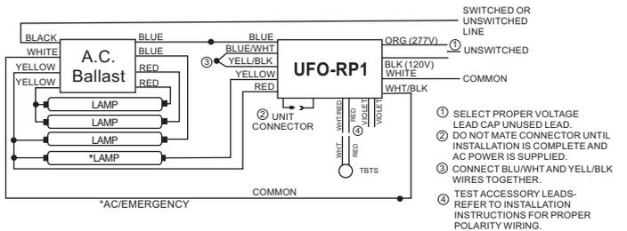
**NOTE: Use the proper input voltage lead, cap unused lead**
