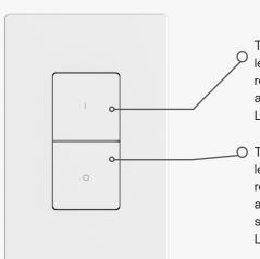
The **ON** function, by factory default, will turn on all relays and raise the dimming level to full for all 16 groups. The user can modify these settings to alter what relays are included with the **ON** function, set a specified dimmer level, and set a specified CCT level if their fixtures are SpectraSync™ enabled through the NX Lighting Controls mobile app.
