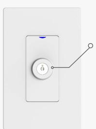
The default operation of the Digital Key Switch is a **TOGGLE** button type with simple 90° right turn for ON/90° right turn for OFF functionality. The user can modify the switch types to be configured to any button type through the NX Lighting Controls mobile app.
