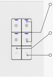
The CCT **PRESETS** 1-4 functions, by factory default, will set the CCT to 5000K, 4200K, 3500K, or 2700K respectively. The user can modify these settings to alter what relays are included with the CCT **PRESET** function, set a specified dimmer level, and enable a Dim to Warm function if their fixtures are SpectraSync $^{\mathsf{M}}$  enabled through the NX Lighting Controls mobile app.
