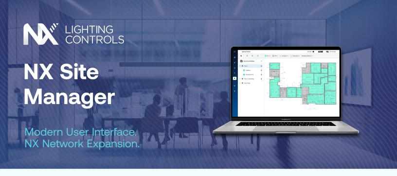
NX Site Manager is a web-based Graphical User Interface (GUI) application for the NX Lighting Control System providing multiple modes of operation, improved facility, user and device management, facility-wide view of schedules, alarms & notifications, and a BACnet/IP interface for connecting to third-party Building Management Systems. NX Site Manager also provides optional add-on applications/features including floor plans with zone status/control, an energy dashboard, and space utilization.
