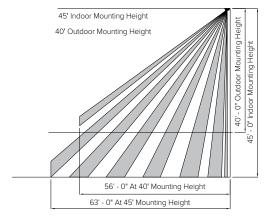
Sensor Lens Coverage and Detection Patterns When Mounted at 40ft and 45ft with Standard Lens
