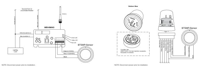
wiSCAPE® Wiring Diagram with WIR-RMI-IO with a BTSMP Sensor
