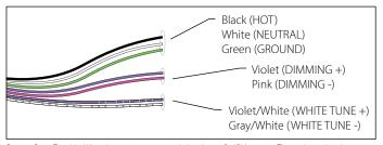
SpectraSync Tunable White luminaires are provided with two 0–10V circuits. The violet and pink circuit is for wiring to any qualified 0–10V controller for dimming. The violet/white and gray/white circuit is for wiring to any qualified 0–10V controller for Tunable White CCT control.
