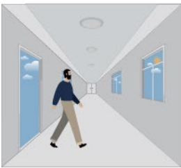
With sufficient daylight, the sensor keeps light OFF even motion gets detected, daylight function is on.
