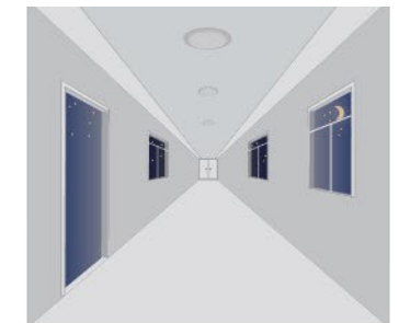
The sensor turns OFF light automatically after the stand-by time when there's no motion detected.
