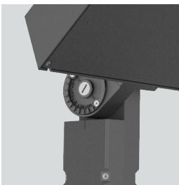
Knuckle – Knuckle mount 15° aiming angle increments for precise aiming and control, fits 2-3/8" tenons or pipes. Available on Area and Flood configurations.
