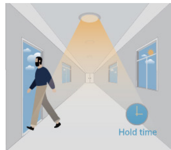
The sensor keeps light ON for hold time after motion leaves.
