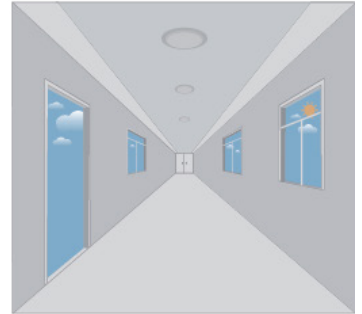
Light OFF when ambient lux level is higher than preset lux amount.
