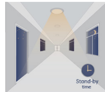
After hold time, sensor dims light to stand-by dimming level for stand-by time.
