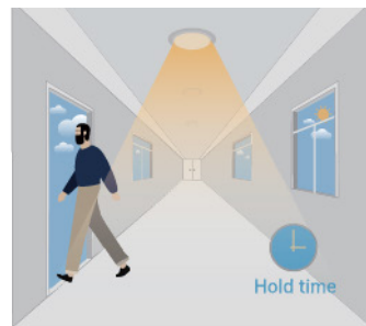
The sensor keeps light ON for hold time after motion leaves.
