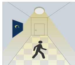
With insufficient daylight, when motion is detected, light turns ON.
